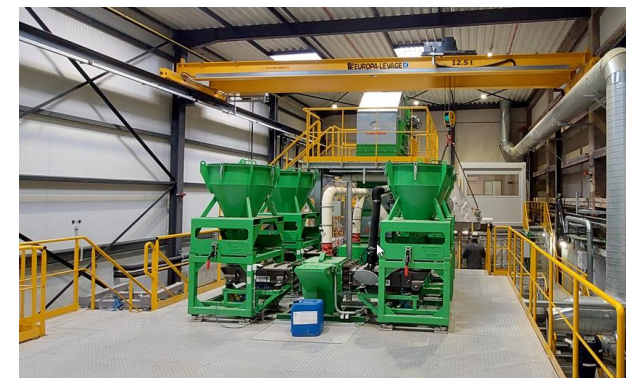
Furnace feeding: Dosing hoppers & conveying system
