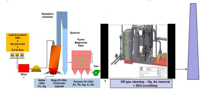
BuLP is a complex material with a high content of sulfur and presence of contaminants: As (0,2-0,4%, Hg (5-20 ppm) that require a dedicated off gas treatment. Nyrstar Hoyanger off gas treatment was designed with BAT techniques:
