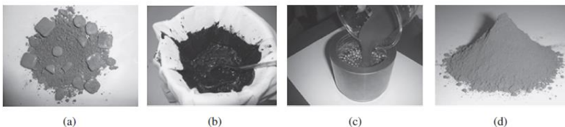
Figure 21: Binder phase removal sequence (a) WC scraps remaining after initial binder phase removal, (b) WC mud after binder phase removal, (c) ball milling (d) dried powder[78]
