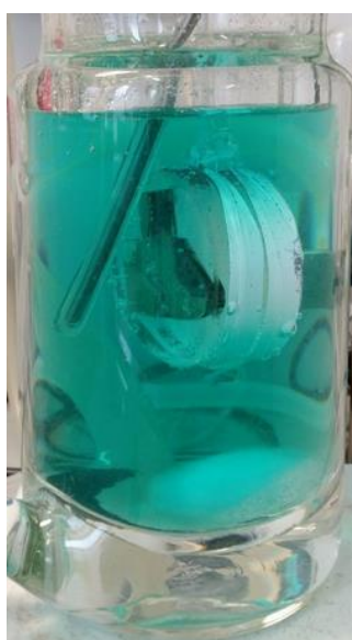
Figure 16: Digestive solution with immersed sample, blue colour indicates digestion of binder material
